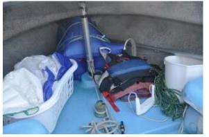
Nine Opti air bags weigh less than seven pounds, cost under \$400 with installation hardware, save skinned shins from sliding into seat edges, and might safe lives. They measure about 32 inches long and 9 inches in diameter when inflated. They still leave room for spinnaker, bucket, paddle, life preservers, and lunch. No downside.
