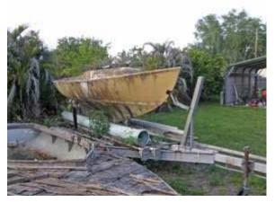
We jacked up the trailer, then removed the wheels and wheel bearings. We fixed the brakes with a Sawzall. We replaced all the wheel bearings and three of the four wheels and tires. One of the replaced wheels was still suitable as a spare. The Sawzall got another workout on a second powerboat trailer that dad found on a tree lawn and dragged home behind his station wagon. The cross-members were rotted, but the wishbone frame was sound. I had ideas of
