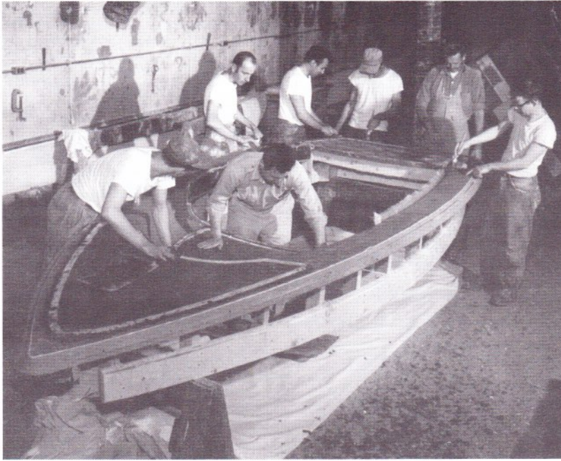
Bullseye deck building in the early 1950's. Seven men! Today this job involves two men clad in OSHA-approved suits and masks.
